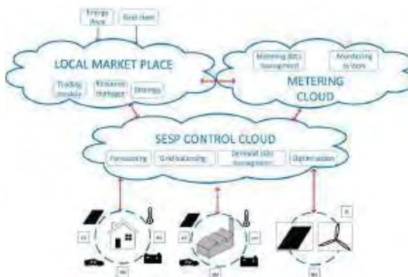
Figure 18: Cloud interactions to facilitate local market operation (Source: EMPOWER D3.2)
