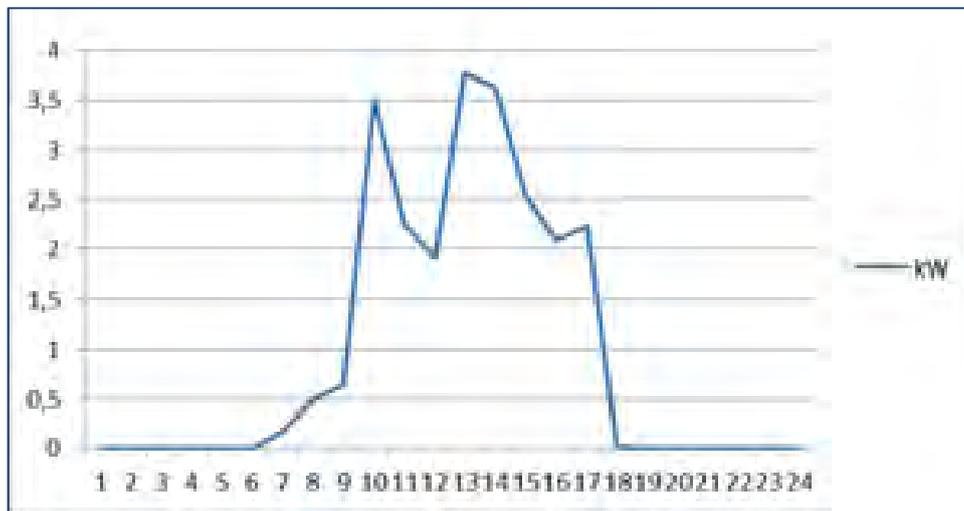
Figure 6: A lightly clouded day yields more irregular generation. Results from a 5 kWp panel
