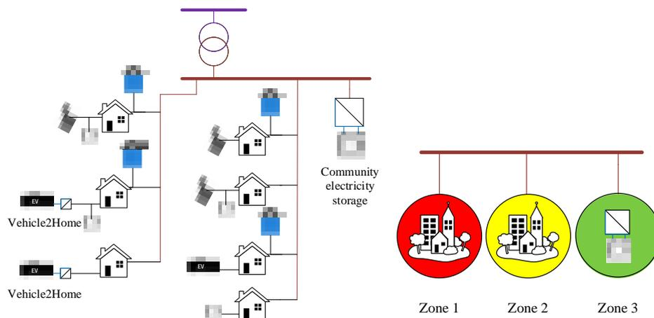
Figure 39: Low voltage distribution grid (Left), Simplified distribution grid in three zones (Right)
