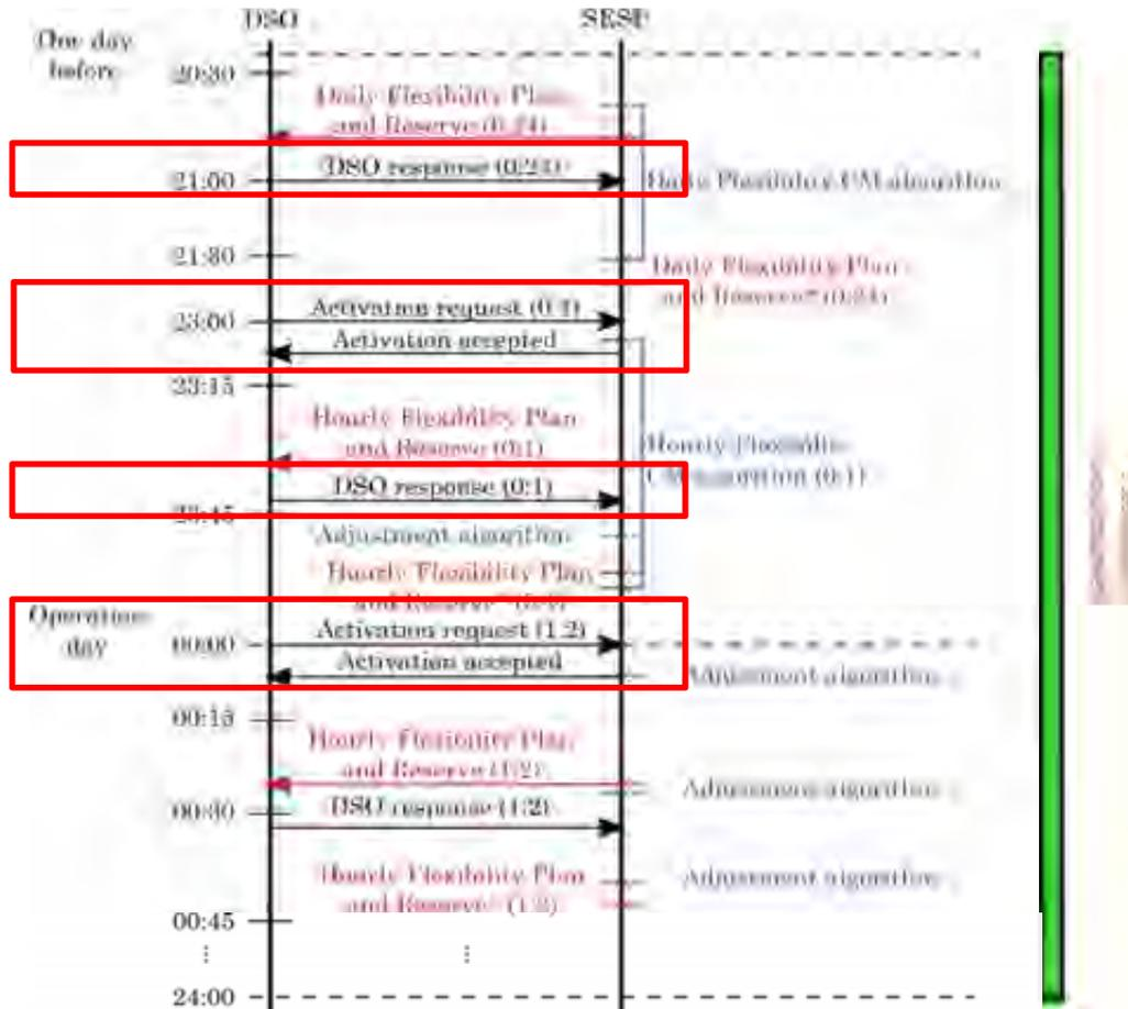
Figure 31: DSO-SESP interactions for supervision LM operation
