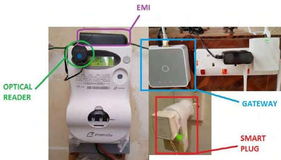
Equipment used at the pilot sites to obtain real time data and control loads
