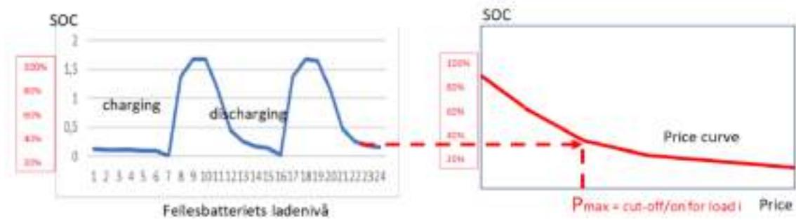
Figure 20: The SOC metering is hooked to the price curve for a community battery, typically in a microgrid setting. Price curve is established based on price limit bids or by the SESP itself. A load or consumer specifies the maximum price that it is willing to opt.
